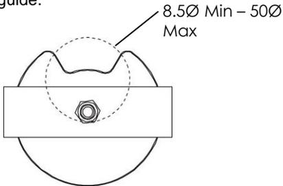
**Step 3.** Place the kidney grommet plate against the bottom of the pole, then put the rod through the desk hole.
