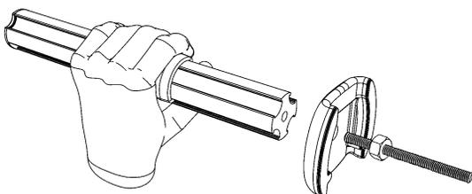
**Step 2.** Fit rubber pads to the top clamp and rest on the table top surrounding the grommet hole with the threaded rod passing through
