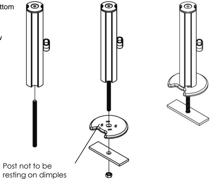
**Clamp assembly - Slimline grommet clamp**
