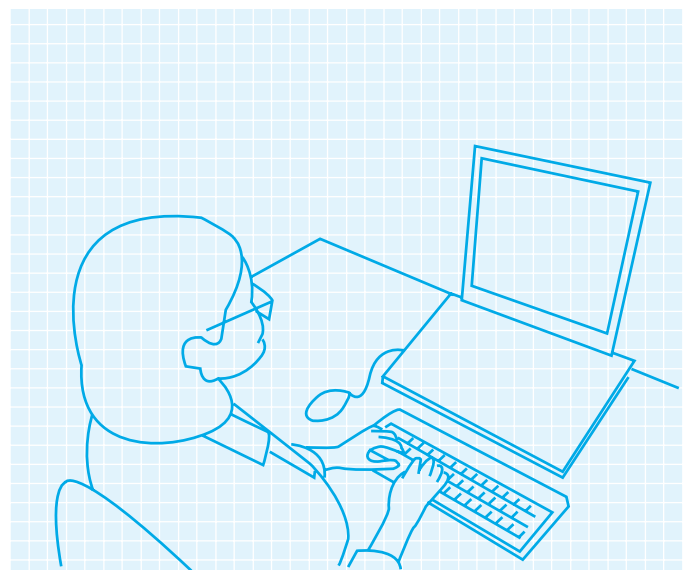
INCORRECT KEYBOARD PLACEMENT: THE ALPHABETIC PART OF THE KEYBOARD IS NOT CENTERED IN RELATION TO THE USER.
